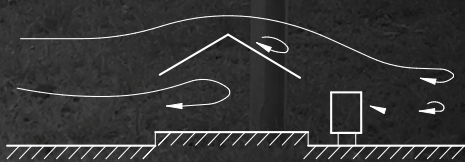
Canopy blocked to the downwind eaves by stored goods ( \varphi = 1 )
